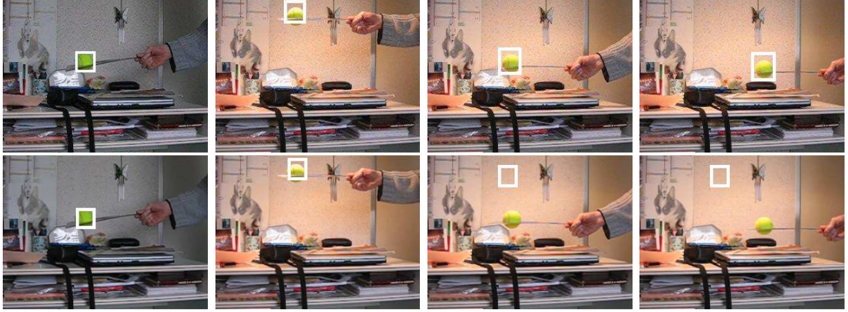
Figure 4: "tennis ball" sequence. Top: successful tracking in presence of an illumination change with HCCS. Bottom: tracking failure with a PF relying on S_{c-t} .
